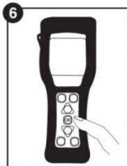
indicate a warning that the surface is not adequately clean. If the reading is greater than 30 the surface is considered dirty.
